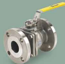
150#, 300#, 600# Flanged Ball Valves Full & Reduced Port Carbon Steel, 316 Stainless & Alloy 20 1/2" - 12"
